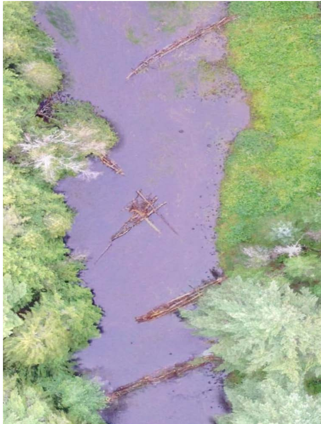
Figure 5.3.4. Aerial drone photo of post-assisted log structures, Outlet 28 Pond, Narraguagus River, Maine, 2017. (credit Carter Stone, University of Maine, Barbara Wheatland Geospatial and Remote Sensing Program)
